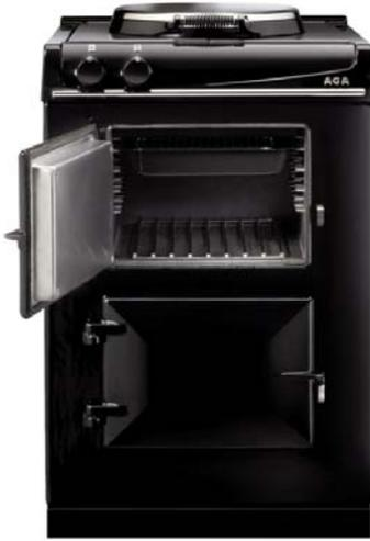
The roasting oven setting is indirectly heated by two elements, one in the base of the oven and the other in the roof. These elements heat the air and the cast iron within to provide cooking results consistent with the traditional AGA heat-storage range, with the flexibility of being able to turn the off when not in use.
