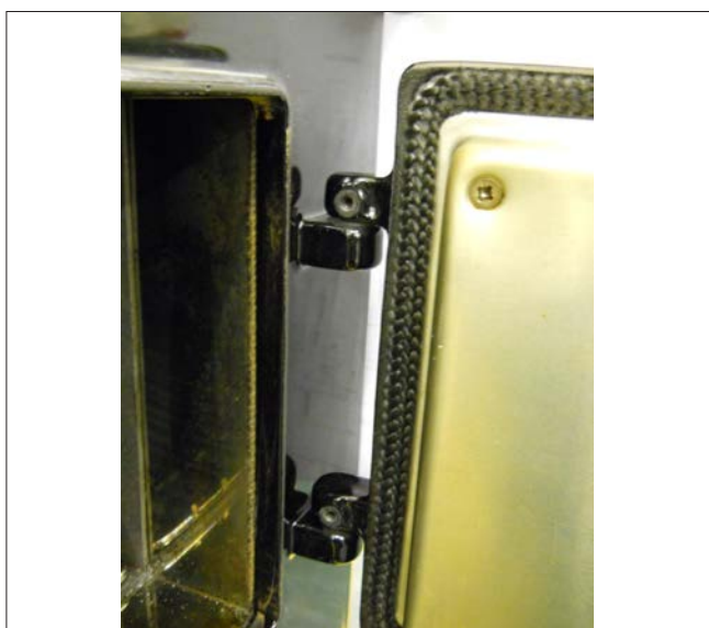
Fig 15 DOOR HINGES LOCATED
