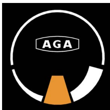
Fig. 3 Amber indicates low temperature setting. (Movement will also be seen with this setting).
